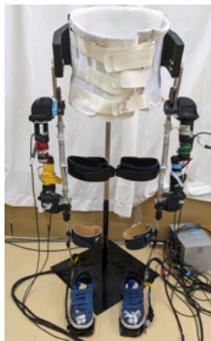
Fig.2 MALO: Motor Actuated Lower-limb Orthosis
