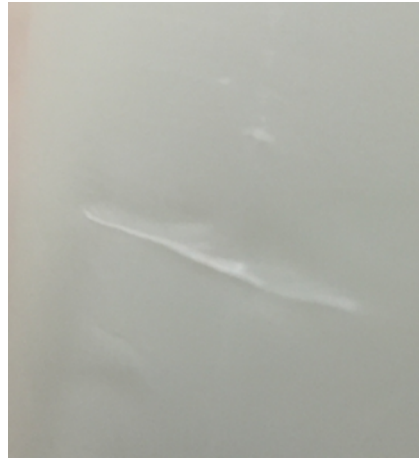
Fig. 4 Surface appearance of dummy skin after abrasion
